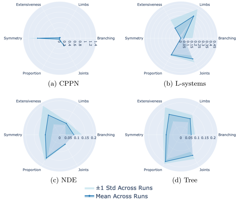
Fig. 8: Radar view of the average 6D descriptors of individuals produced when running evolution with fitness set to 0 for each representation
